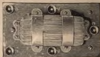
FIG. 262.—Ericsson five-terminal translator for use in multiplex telephone circuit arrangements.
